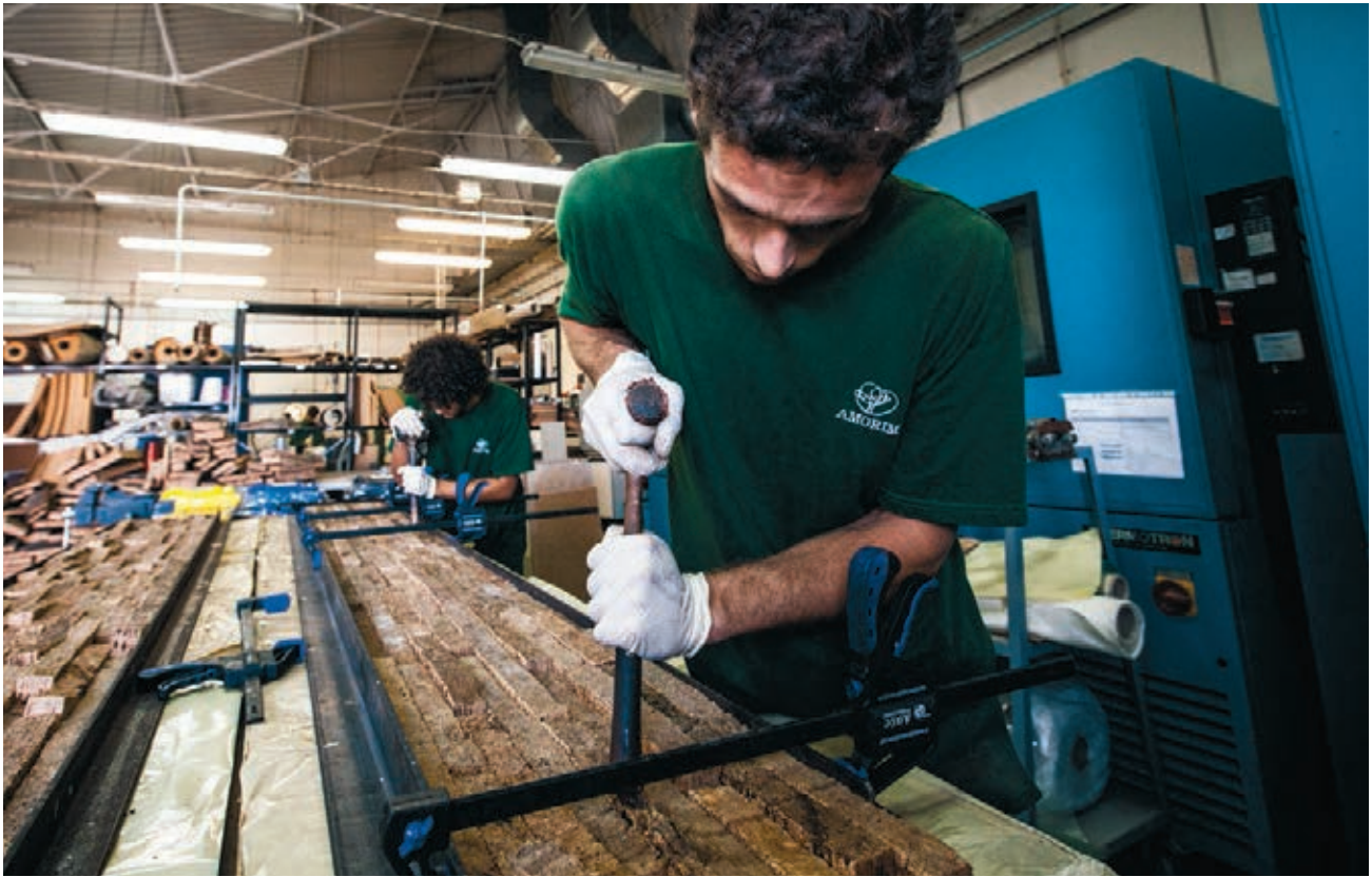
EMPLOYEES OF CORK COMPOSITES BU ARE FINISHING 'SOFT MONOLITHS', AN ARCHITECTURAL CORK SKIN DEVELOPED BY ARCHITECT ALEJANDRO ARAVENA.
