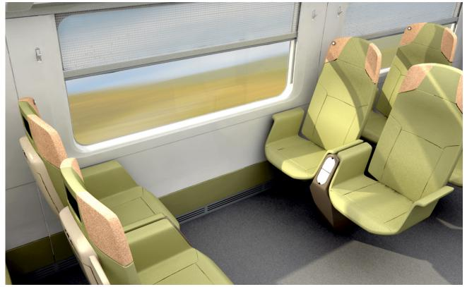
ECOTRAIN PROJECT MAKES USE OF CORK COMPOSITES IN HIGH-SPEED TRAINS
