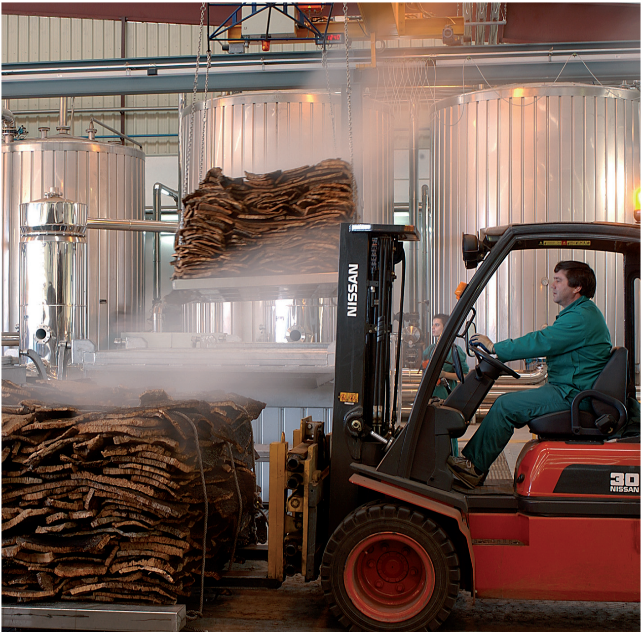
AN EMPLOYEE OF THE RAW MATERIALS BU INVOLVED IN THE OVERALL CONVEX BOILING PROCESS
