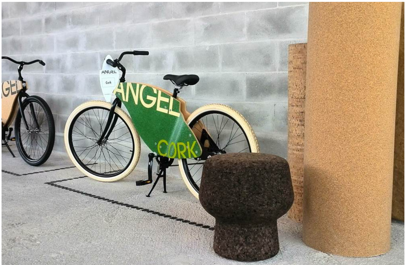
CONCEPT ANGEL, A BIKE MADE FROM WOOD AND CORK COMPOSITES
