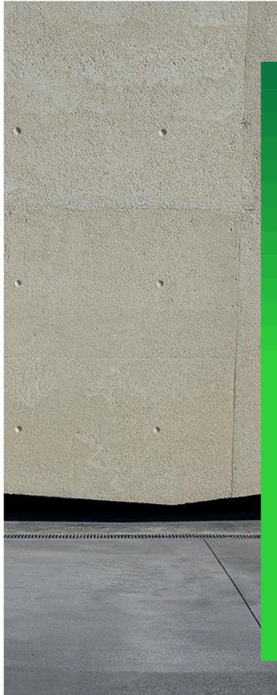
An astonishing soft white concrete, obtained from incorporating cork, which features the lightness and thermal insulation qualities of cork.
