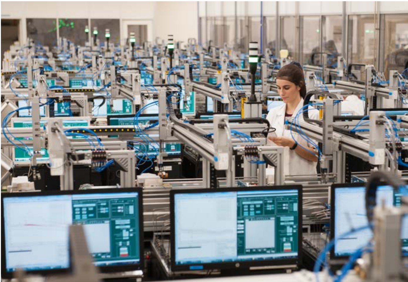
Developed and patented by Amorim, NDtech is an individualized quality control screening technology for natural cork stoppers that delivers the world's first natural cork with a non-detectable TCA performance*. *A non-detectable TCA guarantee means that if any TCA remains in a cork it is below the detection threshold of 0.5 nanograms/litre.
