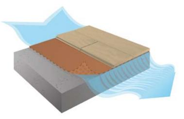
The line of AcoustiCORK<sup>®</sup> products providing acoustic insulation and sound attenuation underflooring for suspended floors is now available in some versions incorporating a membrane insulating against damp.
