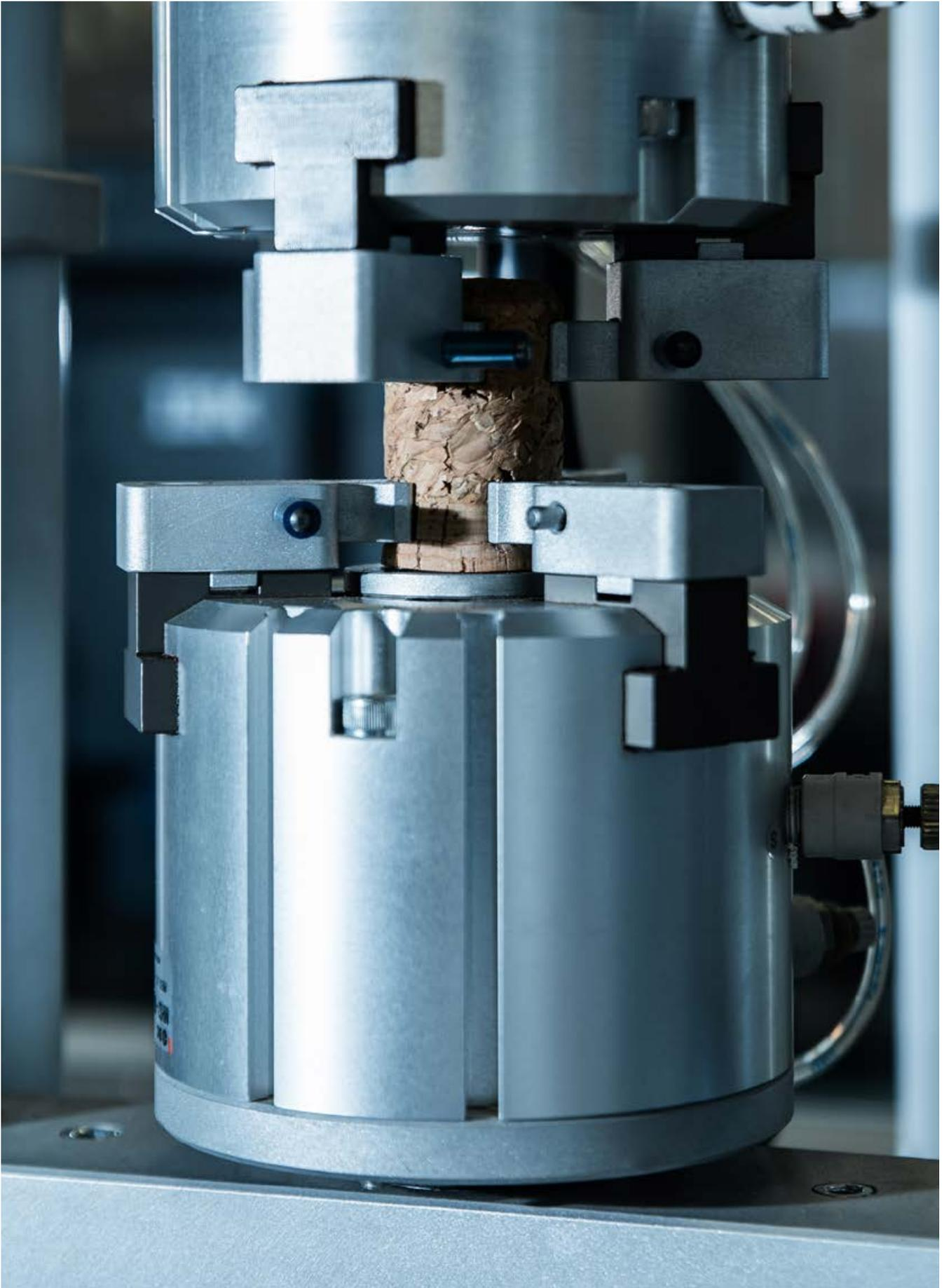
Mechanical test of twisting the stopper for effervescent wines consisting of a body of granulated cork and two natural cork discs.
