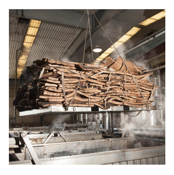
The first selection of cork is followed by a boiling process. The cork planks are boiled in closed and filtered stainless steel tanks. The primary aim is to enable the cork to reach the correct moisture content for processing.
