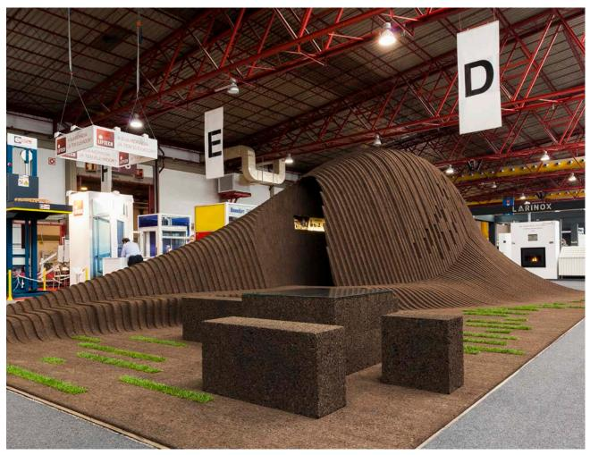
AMORIM ISOLAMENTOS' STAND, TOTALLY MADE OF EXPANDED INSULATION CORKBOARD
