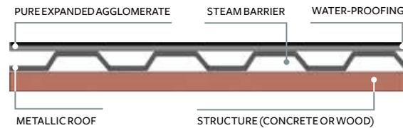
**Image 3** - Use of pure expanded agglomerate in flat roof insulation
