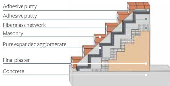
**Image 5** – Use of pure expanded agglomerate in wall insulation (with air cavity)
