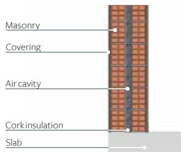
**Image 6** – Use of pure expanded agglomerate in wall insulation
