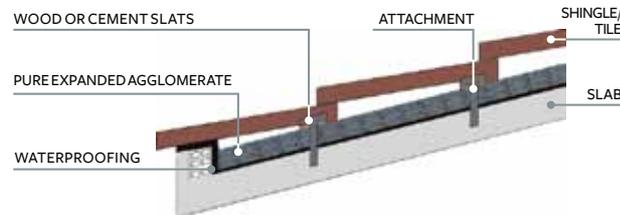
**Image 2 - Use of pure expanded agglomerate in inclined roof insulation**
