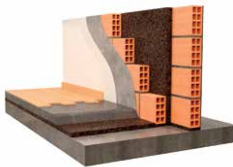
Floating floor with wood covering and Unattached to Wall
