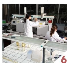
Amorim is a forerunner in strict quality control in each stage of production. Stringent measures also involve the use of a detailed analysis system by GC-MS - Gas Chromatography.
