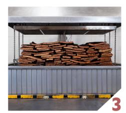
The planks are boiled in stainless steel, closed and filtered tanks. This process softens and cleans the material, while simultaneously expands and improves its internal structure.
