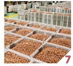
The final stages include: cleaning process with steam distillation, washing in an aqueous hydrogen peroxide solution, polishing and branding.
