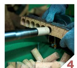
The planks to be used in natural cork stoppers are cut into strips and punched to extract the cylindrical stoppers.
